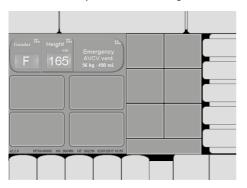
To enter the height, press the **"Height"** button, turn the control wheel to change the value, and press the control wheel to confirm the highlighted option.
