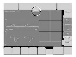
Two cursors (vertical lines) are used to measure and display the values of each curve. The cursor currently selected appears in green.
