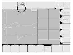
Press kt cancel alarm inhibition. The alarm message remains on the screen.
