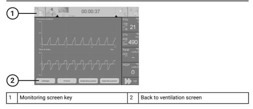
Press the **Ventilation screen** key again or the **Settings** function in the lower left-hand corner to display the ventilation screen with standard monitoring and access to the settings.
