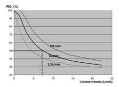
For example, for an O2 supply of 5 L/min and a patient ventilated in volume-controlled mode with a VT of 0.5 L and a frequency of 15 bpm (volume per minute  $0.5 \times 15 = 7.5$  L/min), the maximum obtainable concentration will be approximately 50%. The machine will then be able to supply any desired concentration below this value.
