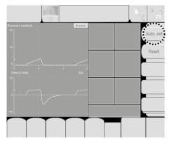
Press the **Auto. set** button, then confirm by pressing the rotating knob: all of the alarm thresholds update automatically.
