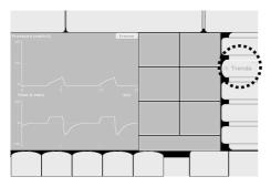
The trend curves can be displayed for 5, 20, 40 or 80 hours. To change the time scales, press the **zoom** + or - buttons.
